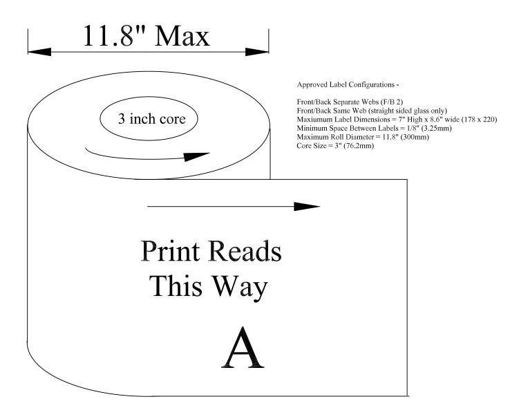
Labels are Outside Wind, Right Off. Unwind Direction #3
